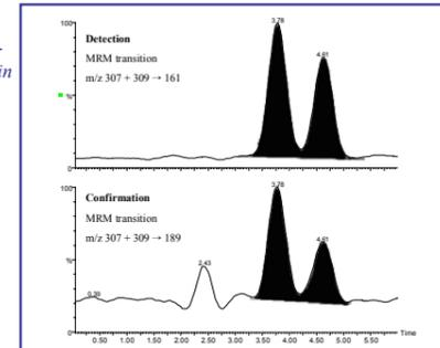
of detection was determined experimentally to be approximately 0.007  $\mu$ g/ml, equivalent to 0.3 mg/kg in liver tissue (fig.7). This is well below the usual residue range (5-130 mg/kg) in liver tissue associated with fatal poisoning. Evidence for the confirmation of residues was provided by the simultaneous acquisition of data from an alternative
