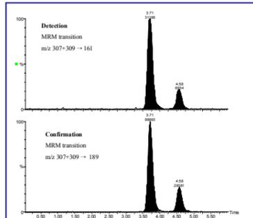
Figure 9. Detection and confirmation of a chloralose residue (5.2 mg/kg) in liver tissue from a buzzard.
