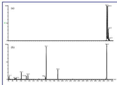
Figure 5. Reconstructed ion chromatograms illustrating effect of solvent (precursor ions m/z 307 + m/z 309  $\rightarrow$  product-ion m/z 161), for chloralose standards (1.5  $\mu$ g/ml). Matrix concentrations equivalent to 0.025g/ml.
