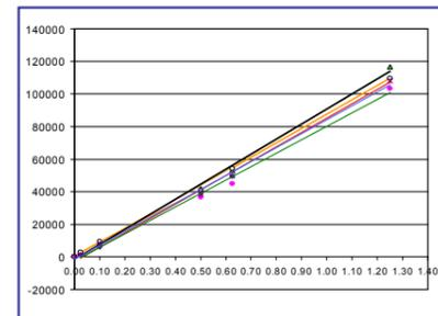
from standards in pure solvent (fig.6) was linear over the range 0.02 to 1.3  $\mu$ g/ml. Tests on standards made up in matrix extract solutions demonstrated that calibration was essentially free from adverse effects from matrix components (fig.6). Recovery experiments on fortified tissues were performed using calibration against standards prepared in
