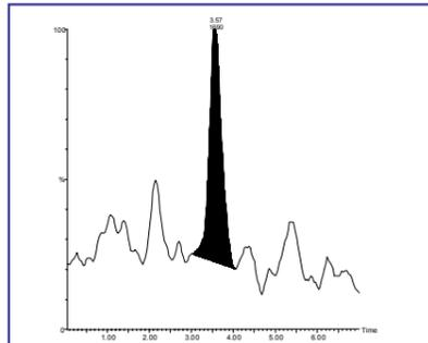
Figure 8. Detection and confirmation of a chloralose residue (1203 mg/kg) in a sample of material recovered from the gullet of a buzzard.
